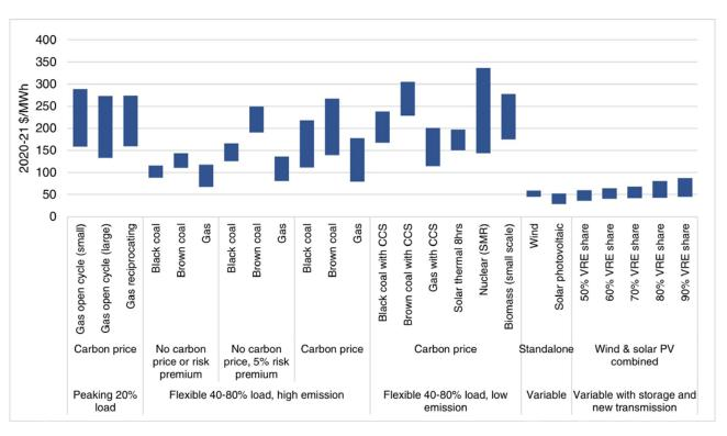
FIGURE 04: Calculated Levelised Cost of Energy by technology and category for 2030
